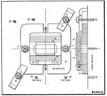
Fig. 44. Form of Die-bed adapted to General Use
